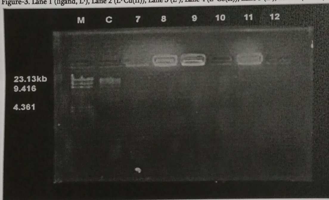
Figure-4. Lane 7 ( L^8 ), Lane 8 ( L^8 Ni(II)), Lane 9 ( L^8 Cd(II)), Lane 10 ( L^8 Zn(II)), Lane 11 ( L^8 Hg(II)), Lane 12 ( L^8 Fe(III))
